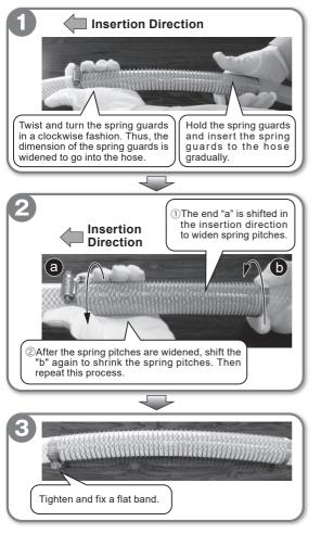
When installing the spring guards, hold the end of the spring guards by hand. Turn the flat band in a clockwise fashion and insert the spring guards, keeping the spring diameter widened.
