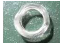
↑ 八興 E-SJ-4×6 HAKKO E-SJ-4×6 ● 試験回数 : 100 万回 Number of Attempts : One Million Times
